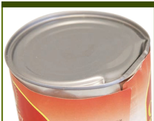
Severe dent in seam
