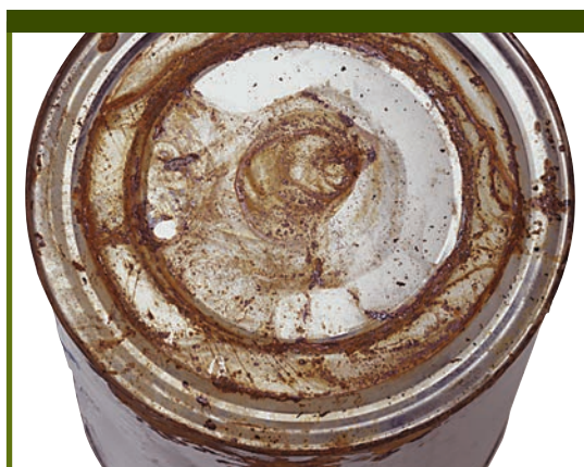
Rust that cannot be wiped off
